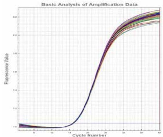
Simultaneous scanning of the six-channel shows that the standard deviation of the Ct value of the FAM channel is <0.07. No fluorescence signal in other channels.
